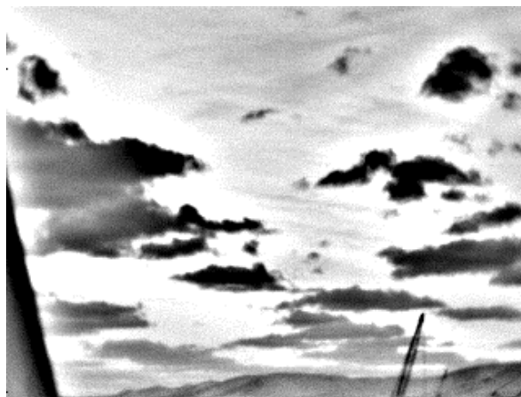
Figure 1.24 A cloud image taken with a Raytheon Series 2000B camera from the top of the physics building in Adelaide - looking north-east. It's a pyroelectric 320 \times 240 pixel camera sensitive to 7\text{-}14\mu\text{m} infra-red radiation. A negative image is shown - dark (cloud) areas are warm compared to white (clear sky) areas. The image shows cumulus cloud low over the Adelaide Hills - at least 10 km distant. Some closer cumulus is evident in the middle of the image. This foreground cumulus is in front of some higher altitude diffuse/cirrus type cloud (faintly visible in the upper centre of the image). On the left is part of the physics building and in the lower right a construction crane. The horizon is the Adelaide Hills.
