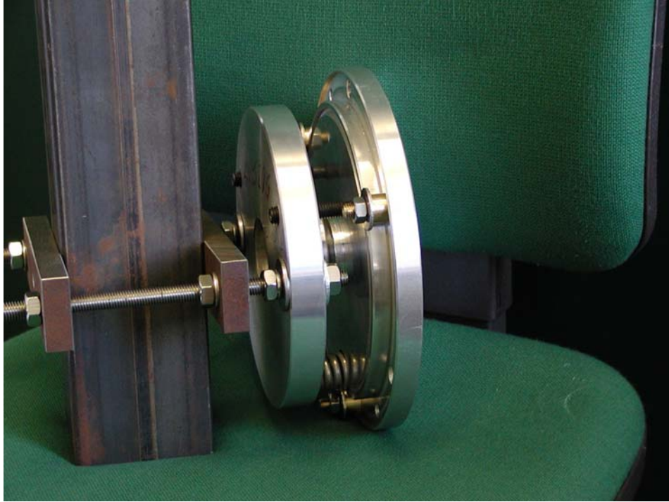
Figure 1.9 Photograph of a new prototype of the mirror mount to be used with both the aluminum and glass mirrors.
