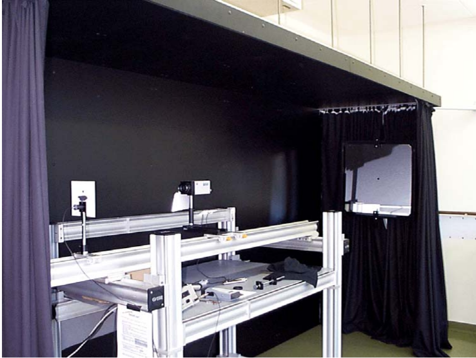
Figure 1.5 An aluminum mirror element mounted on an optical test stand for the determination of the effective optical properties – radius of curvature and the intensity distribution of the reflected light.
