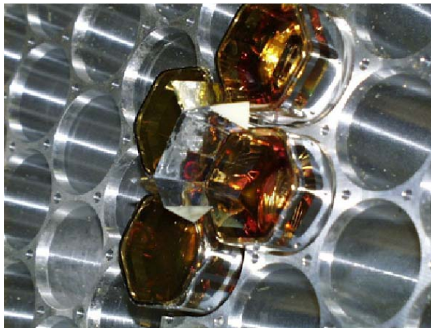
Figure 1.16 The mounting of light collectors.
