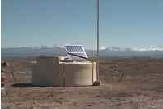
Figure 2. Picture of a water Cherenkov tank installed on the site. The solar panel and the antenna are visible
