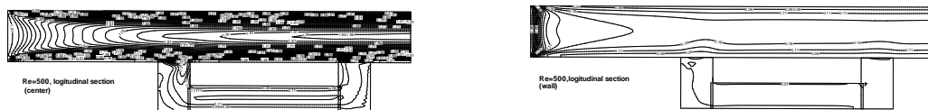
Fig. 5, 6: Isolines of velocity in angular bypass for Re = 500 , 3D case in the central plane xy , 3D case in the xy plane near the wall.
