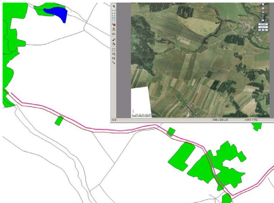
Fig. 5 Example of data sources used in the “Gap Analysis” – digital aerial orthophotographs and maps of scale 1:25 000
