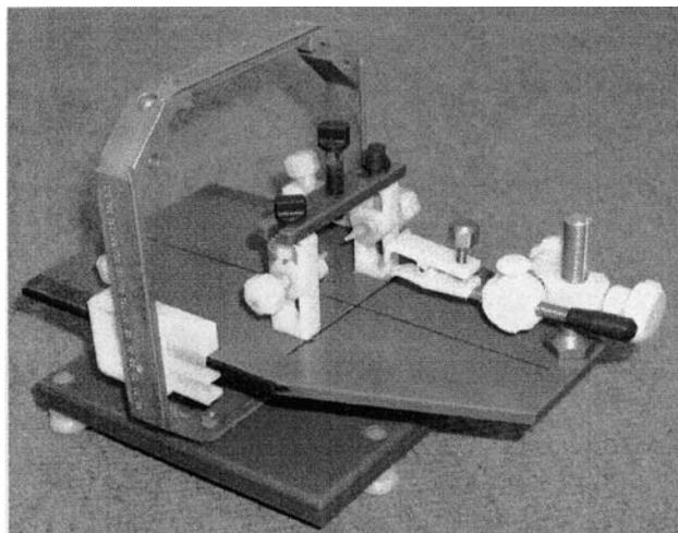
FIG. 1. Photograph showing the stereotactic MR imaging-compatible apparatus for rat fixation.
