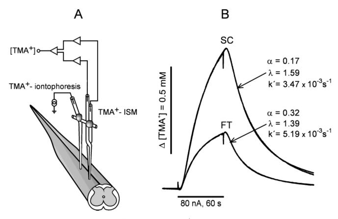
Fig. 2. Experimental set-up and representative diffusion curves obtained in the spinal cord and filum terminale. A: The experimental arrangement. A TMA<sup>+</sup>-selective double-barreled ion-selective microelectrode (ISM) was glued to an iontophoresis microelectrode. The separation between electrode tips was 100–200  $\mu$ m. When the electrode array was inserted into the spinal cord and the iontophoretic current applied, the diffusion curve resulting from the increase in
