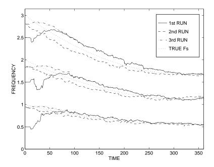
The performance of the MFT algorithm on a three component quadratic frequency-modulated signal embedded in a white Gaussian noise. SNR=-5dB for all three components. The first (forward) run of MFT is used to achieve convergence of the algorithm to true frequencies, because the true initial frequencies are not assumed to be known. The second (backward) and the third (forward) runs of MFT are used to estimate the polynomial phase parameters.
