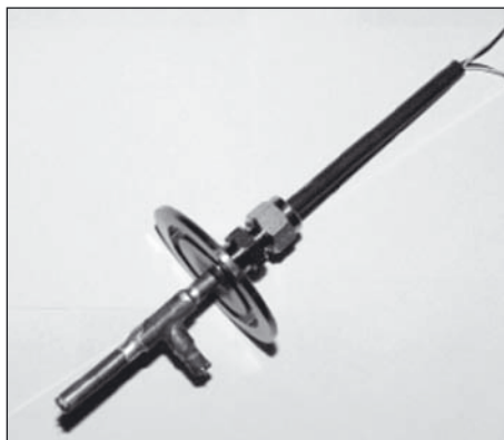
Fig. 5 Special grommet for temperature sensor
