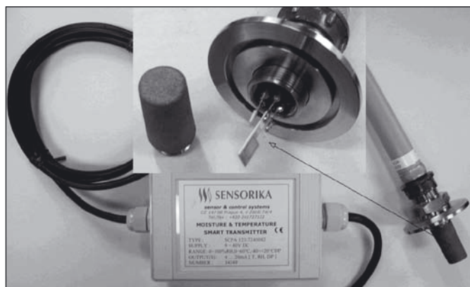
Fig. 6 Probe HTP-25 incorporated in the Sensorika humidity sensor
