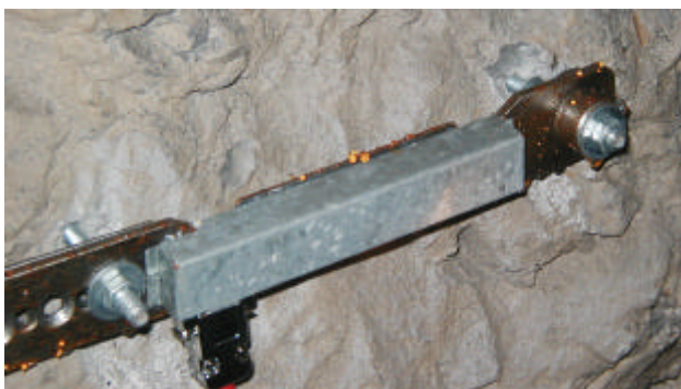
LA04. Portable 4-channel unit with display and RS485 interface; application in harsh environment (tunnel Višòové)
