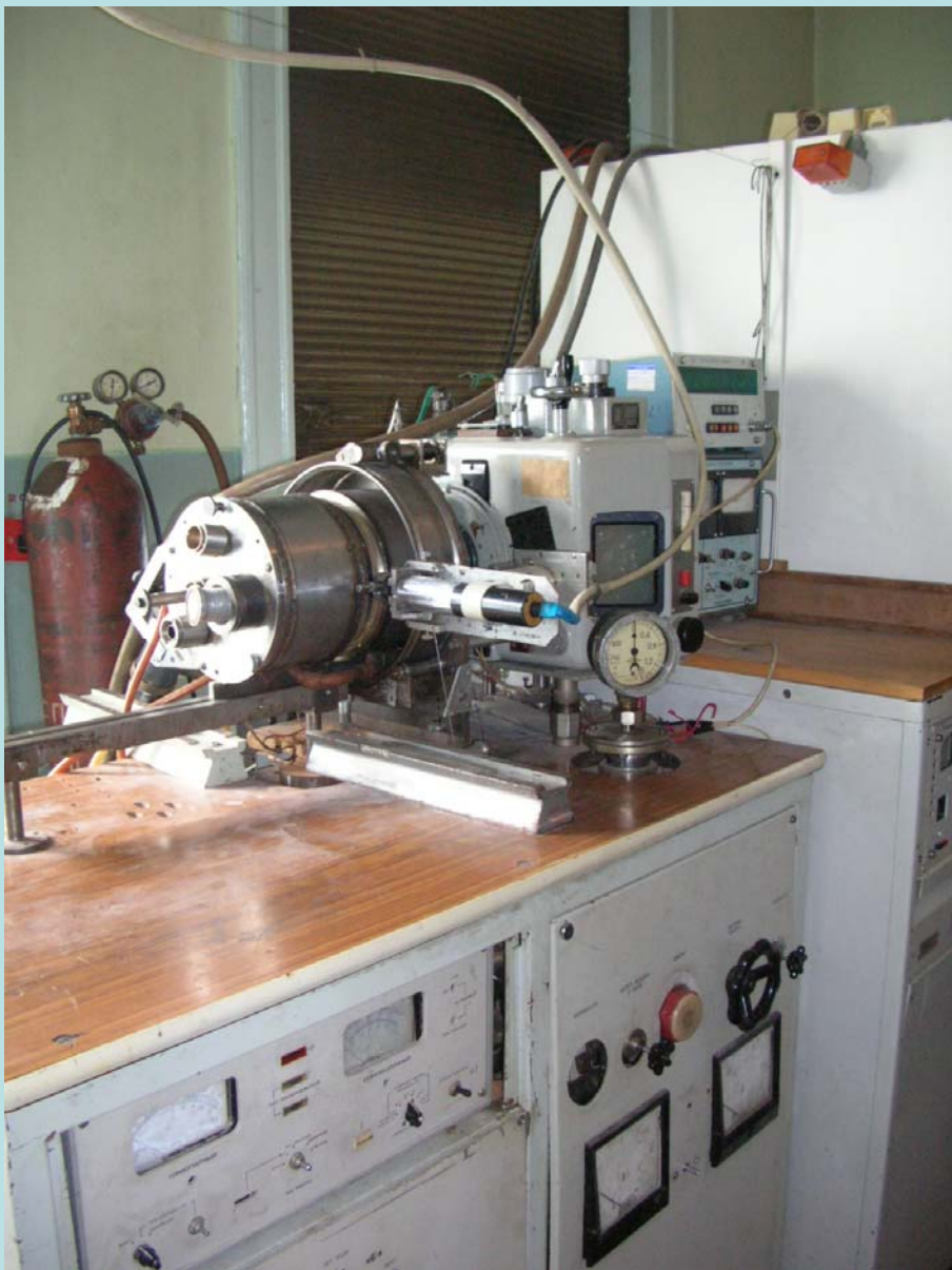
High-temperature X-ray diffractometer with horizontal axis
