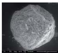
Figure 2- SEM analysis of chitosan-D2HEPA microcapsule cross-section
