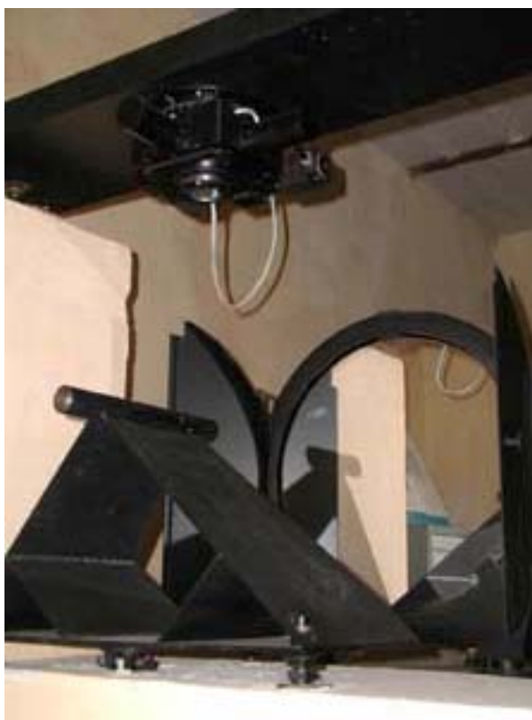
Fig. 8: Guiding telescope, table of the coordinate system with the guiding sensor, and the primary mirror (objective) of the telescope. The construction of the coordinate-system table enables a scanning of an arbitrary rectangular region on the solar disk and in its near surroundings (including a scanning of a region inclined by a given angle with respect to the axis of solar rotation).
