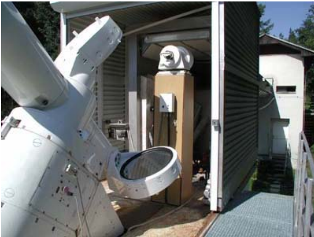
Fig. 4: The main and auxiliary mirrors of the Jensch-type coelostat with the control panel. The secondary mirror of the telescope with a focussing system is located on a top of a column in the center of the picture.
