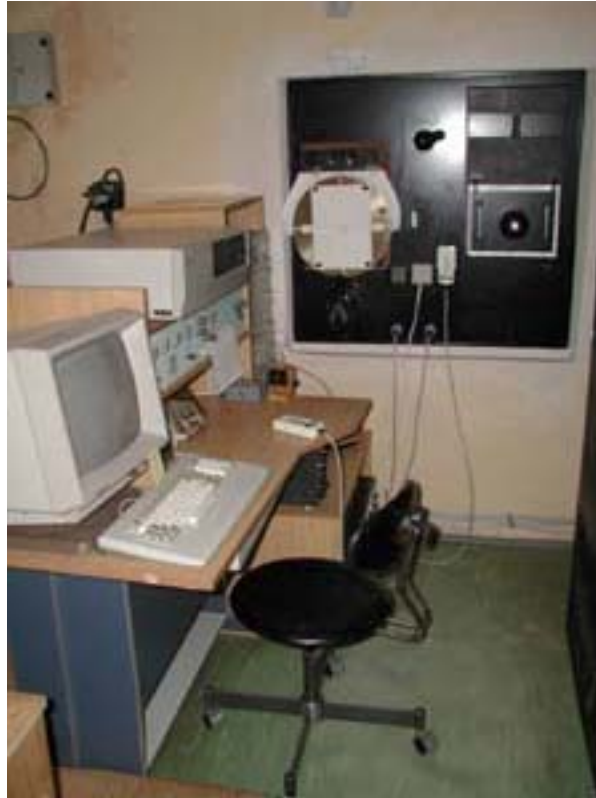
Fig. 2: Front wall of the spectrograph with a screen in the telescope's focal plane (the full solar disk can be projected) and with the entrance slit in the center of the screen. The old control panel of the magnetograph is seen on the left.
