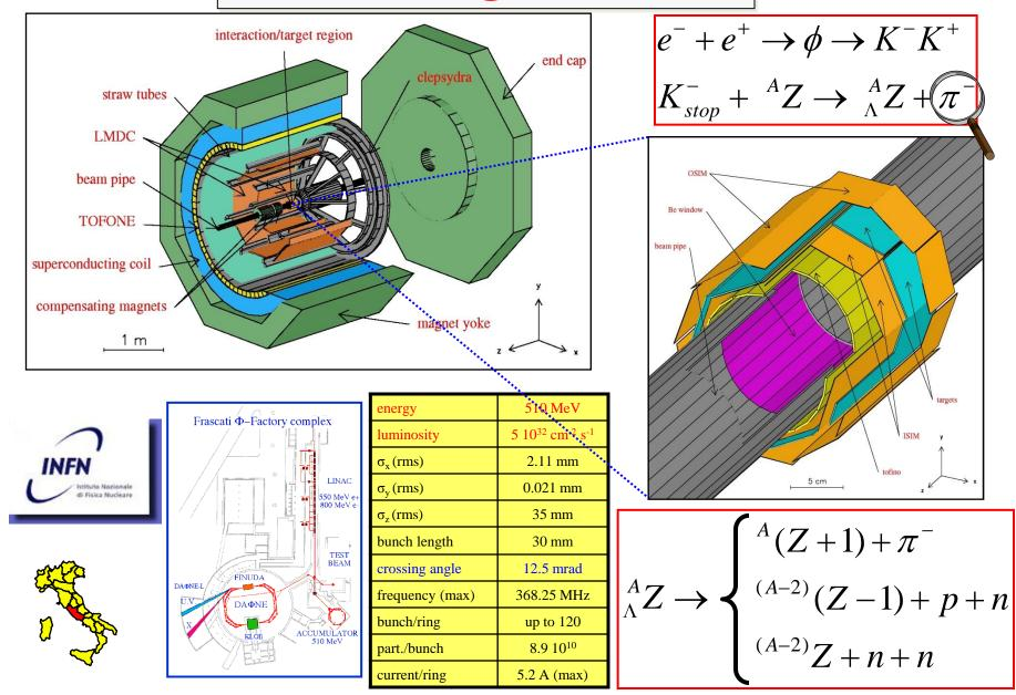
Last evolution of the  $K_{stop}^-$  approach  $\Phi$ -Factory  $\rightarrow$  Source of Low Energy  $K^-$  (~16 MeV) – Thin targets
