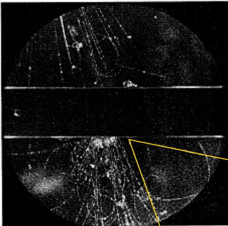
First cloud chamber photograph of a neutral  $\Lambda$ -particle. Obtained by G. D. Rochester and C. C. Butler at the University of Manchester, the  $\Lambda$ -particle was produced in a 3-inch thick lead plate and decayed into two particles identified by the arrows labeled 1 and 2 at the edge of the figure. (Reproduced through the courtesy of Nature.)
