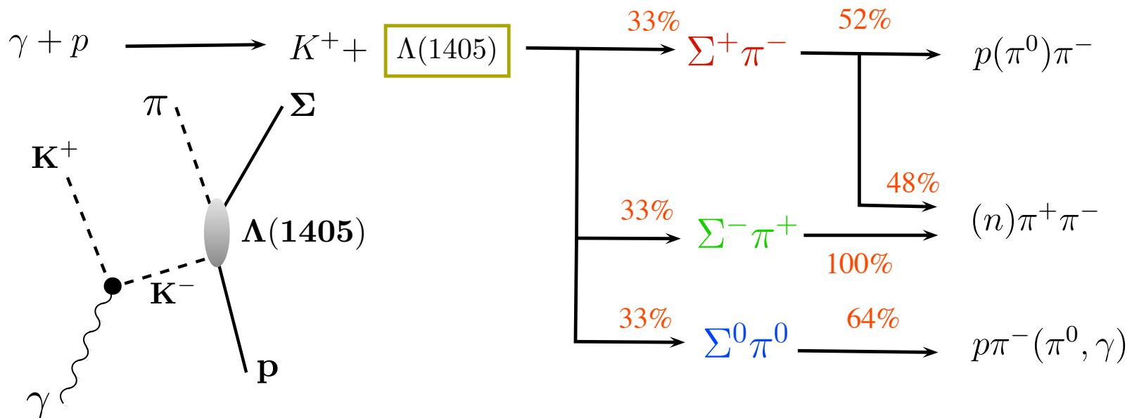
$$\frac{d\sigma(\pi^+ \Sigma^-)}{dM_I} \propto \frac{1}{2} |T^{(1)}|^2 + \frac{1}{3} |T^{(0)}|^2 + \frac{2}{\sqrt{6}} \text{Re}(T^{(0)} T^{(1)*}) + O(T^{(2)})$$
