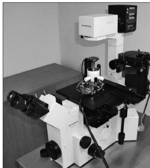
Fig. 2 AFM Explorer on the preparation table of inverted light microscope Olympus IX 70
