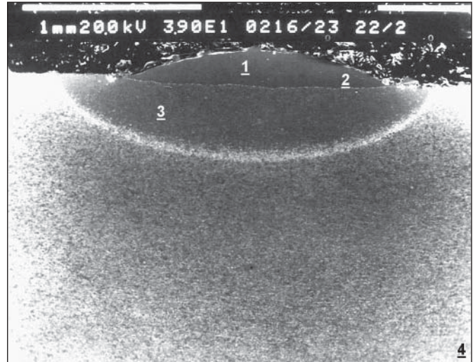
Fig. 10 Structure in the cross-section of laser surface treated layer on steel ČSN 41 1373 (1 - the clad layer, 2 - transition zone, 3 - heat affected zone of base material, 4 - non-affected base material)
