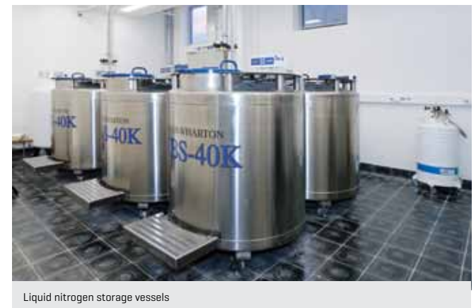
Liquid nitrogen storage vessels
