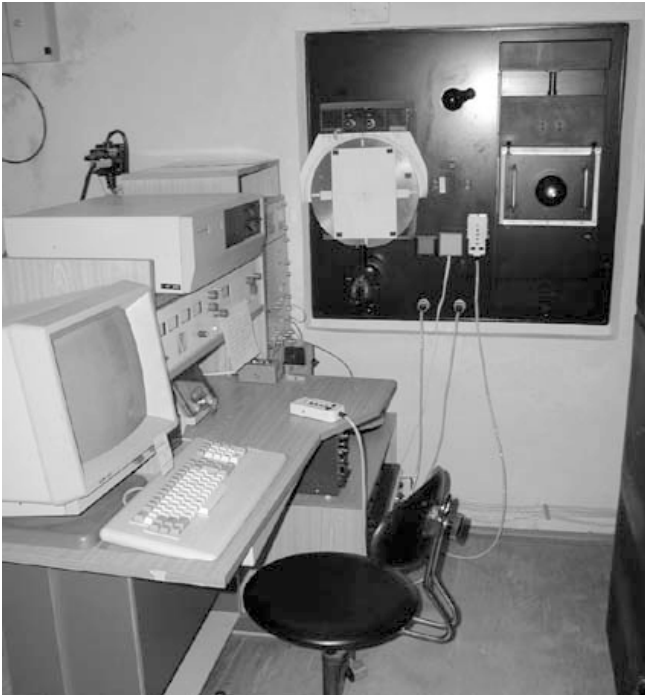
Fig. 3. Front wall of the spectrograph with a screen in the telescope focal plane (the full solar disk can be projected) and with the entrance slit in the center of the screen. The old control panel of the magnetograph is seen on the left.
