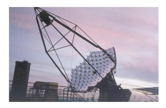
SIMAX was used as mirror substrate. This idea is know-how of our laboratory. The SIMAX is comparable to more expensive PYREX glass that is usually used for similar applications. The mirrors had the diameter 500 mm and the thickness 11 mm. We simulated the distortion of the mirror segment by gravity in wide
