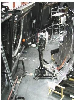
We changed our original circular mirrors with diameter of 500 mm into quasi-hexagonal shapes with the larger size at the same time. The hexagons cover the main mirror better than circles. The light losses are eliminated. Our new hexagonal type of mirrors has thickness 17 mm and circumscribed diameter over 600 mm.
