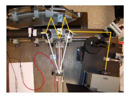
Next advantage is that we are able to change beam wavelength and measure the dependency of reflectivity on wavelength. Some results from our measurements are shown in the next graph.
