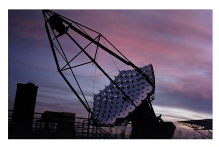
Mirror has surface 16 square meters and is composed from 90 segments. One mirror segment has diameter 500 millimeters and radius of curvature 12 meters. Camera in focus is compound from 546 photomultipliers Hamamatsu, one pixel has 13 millimetrs in diameter and resolution is 2,2 mrad. CAT aims on particles with energies 180 – 2000 GeV. We enter the project in 1994 and from 1997 is telescope in full duty.
