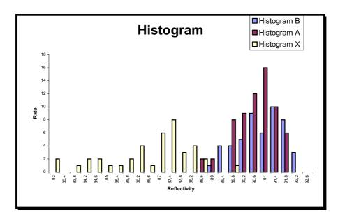
Homogeneity of reflectivity over the whole surface lies in 2,5%. This differences are caused by evaporization process, where the mirror is rotating along own axis and the vaporization source of aluminum and silicon dioxide is point.
