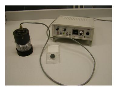
The measurement is based on comparing of voltage on photodetector with calibrated mirror with reflectivity 90,6% on 375 nanometers and measured mirror. This is simple and functional method.
