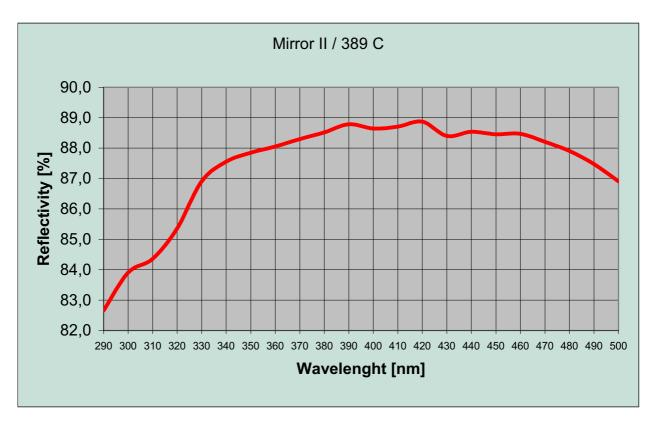
Average reflectivity of 60 mirrors for one telescope is 90,5% for telescope A, 90,7% for telescope B and 90,8% for telescope C in the UV region (375 nanometers). Next graph shows histogram of reflectivity for prototype and for first two produced telescopes.
