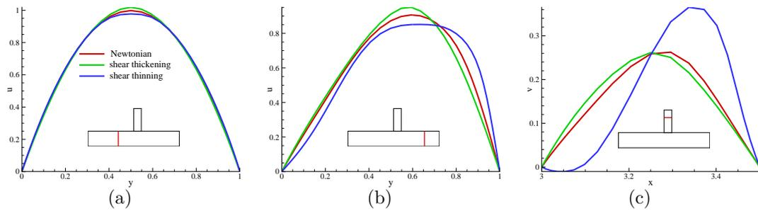
Figure 3: Nondimensional velocity profile for steady fully developed flow of generalized Newtonian fluids in the branching channel.
