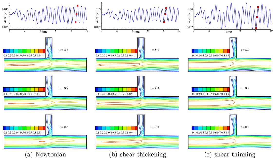
Figure 4: The graphs of the velocity as the function of time and velocity isolines of unsteady flow of generalized Newtonian fluids by artificial compressibility method (frequency is 2).
