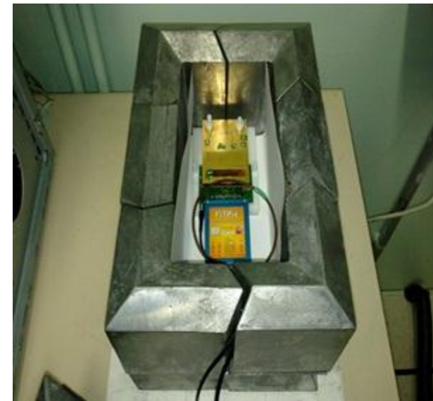
Measurement setup with 5 cm lead shielding
