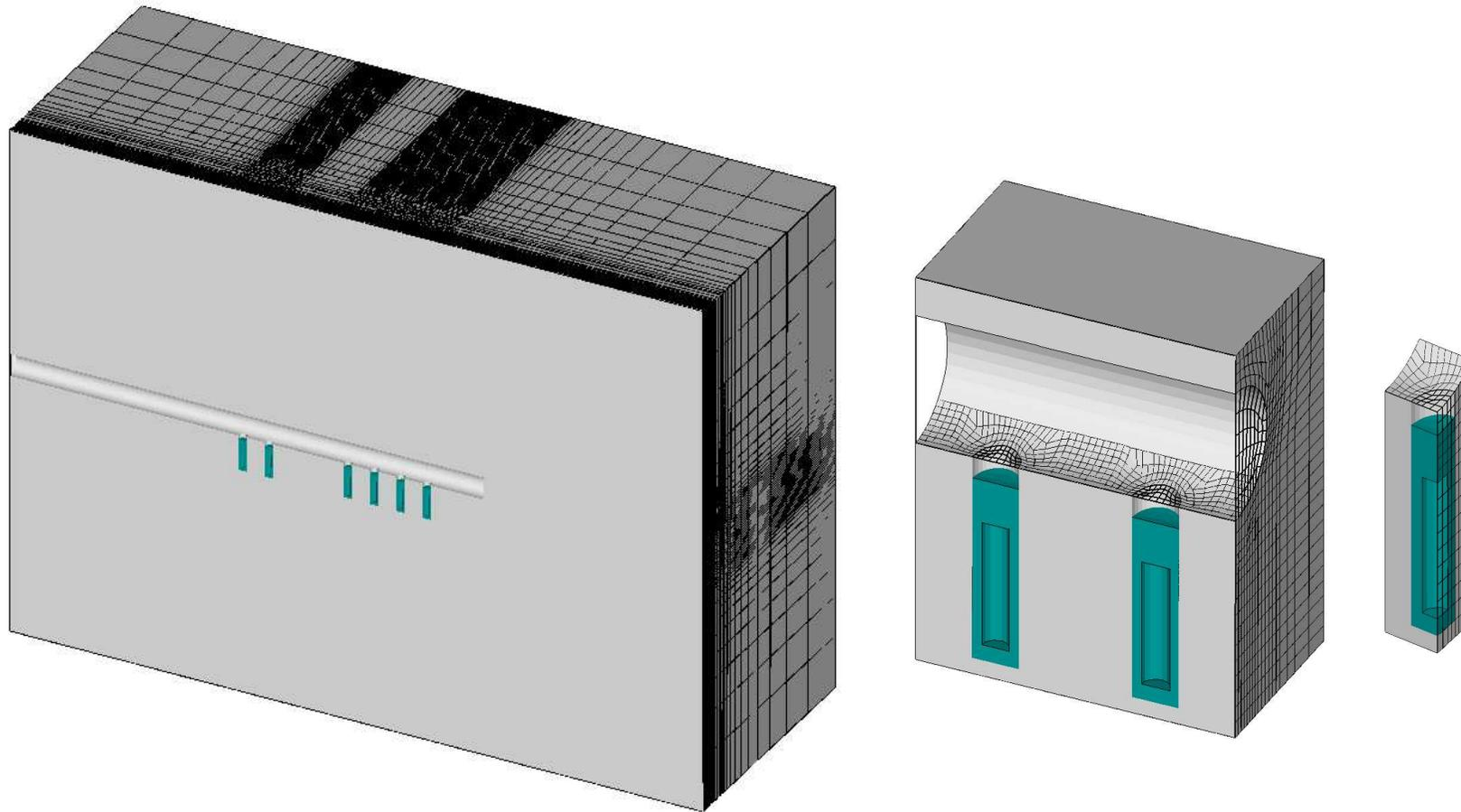
Linear tetrahedral FE (15 mil. tetrahedra),  $>2.5$  mil. DOF for heat transfer,  $>7.5$  mil DOF for elastic displacements, time period 50 years.
