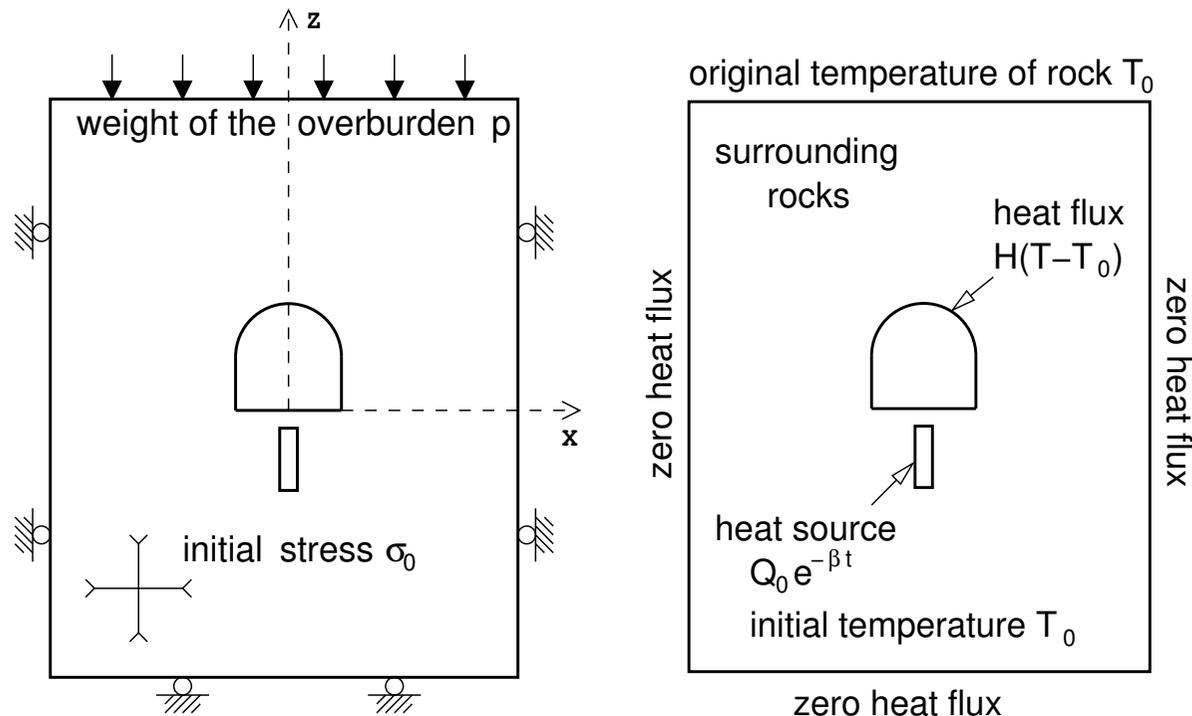
FEM discretization in space, FD discretization in time: *find nodal temperatures  $\tau^k$  and nodal displacements  $u^k$  in time steps  $t_k$*
