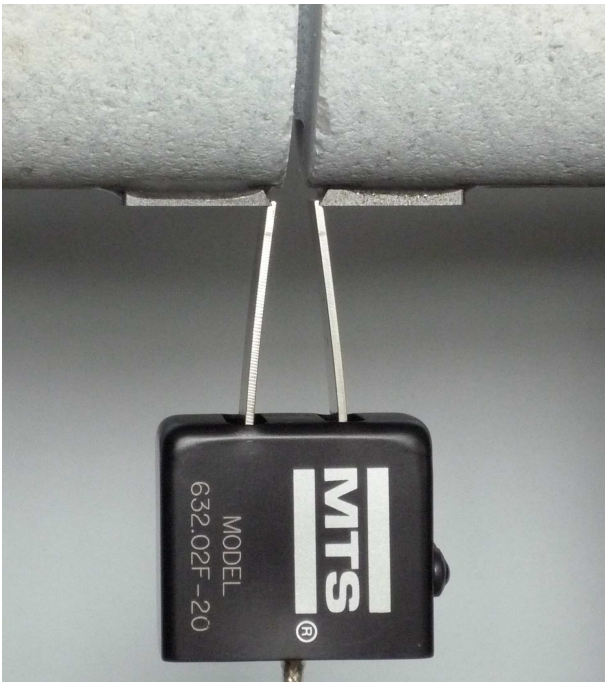
Figure 3: The clip on cage (close-up), type of extensometer
