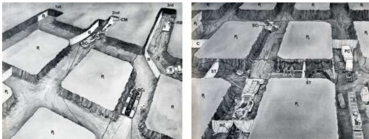
Obr. 1 Metoda KOMORA-PILÍŘ, CM -Continuous Miner, SC 1 -Shuttle Car, RB -Roof Bolter, S - Scoop, B -Brattice, PC -Power center, F -Feeder, B -Breaker, BC -Belt Conveyor, ST -Stopping, T -Track, MT -Man Trip, P 1 -Pillar (Peng, 2008)
