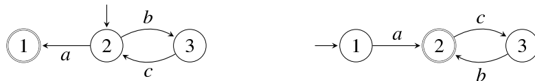
Figure 8: SPA G (left), and DFA G^R for the reversal of the language L(G) (right); projection P : \{a, b, c\}^* \rightarrow \{a, c\}^* .
