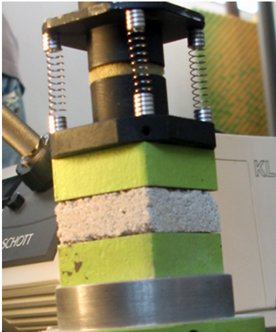
Measured compression strength dependence on the slenderness ratio
