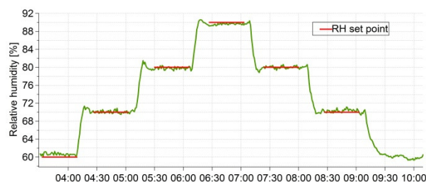
Figure 1: RH control of aerosol conditioning system ACS
