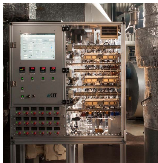
Figure 1. HICE exposure system for air-liquid interface exposure of human lung cells towards combustion derived particle emissions
