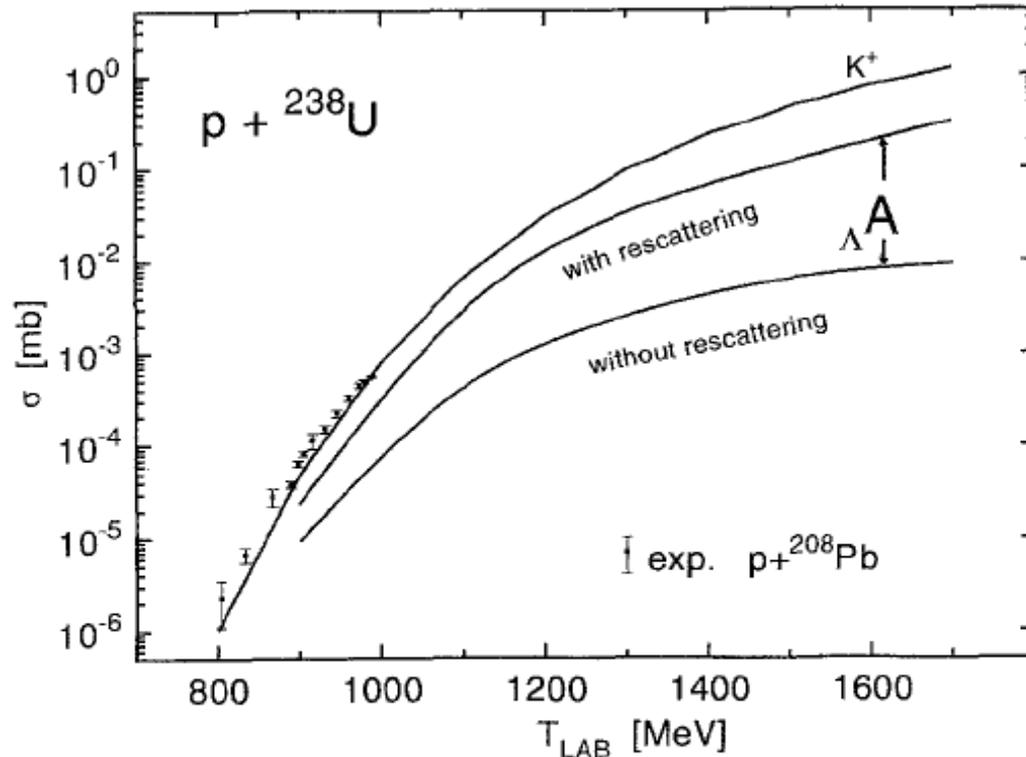
**Fig. 5.** The energy dependence of the  $\Lambda\Lambda$  production cross section for the cases with and without  $\Lambda$  hyperon- $N$  rescattering. For relative orientation we also compare the calculated total  $K^+$  cross section with the inclusive  $K^+$  data from [30] for  $p + {}^{208}\text{Pb}$
