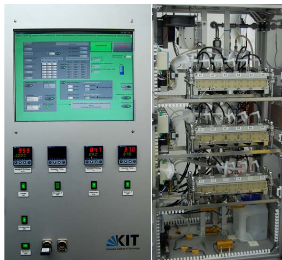
Figure 1. HICE exposure system for air-liquid interface exposure of human lung cells towards combustion derived particle emissions
