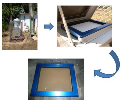
Figure 1. The PM 10 samples were collected using high-volume sampler in Porto Velho, Amazon region.
