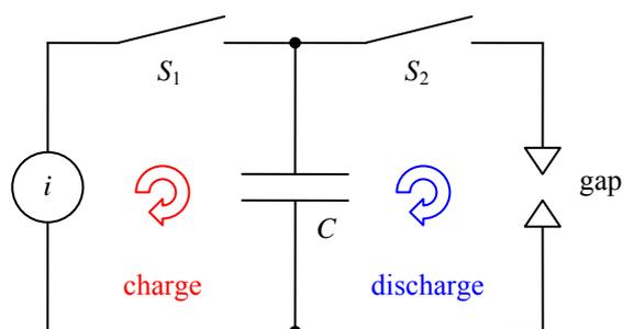
Figure 1. New spark generator concept
