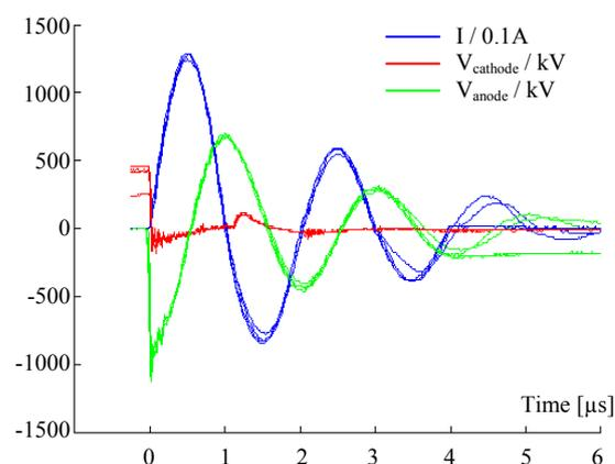
Figure 2. Oscilloscope traces of 9 consecutive 1.2 kV, 32 mJ sparks at a 6.6 kHz repetition rate.
