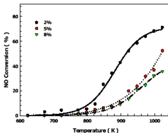
Figure 1. Effect of various copper loading on the nanosized Cu/ $\gamma$ -Al<sub>2</sub>O<sub>3</sub> catalyst for the conversion of NO with CH<sub>4</sub>. Test conditions : 600 ppm NO in He, 600 ppm CH<sub>4</sub> in He, O<sub>2</sub> = 2%, GHSV = 108000 ml/h-g.
