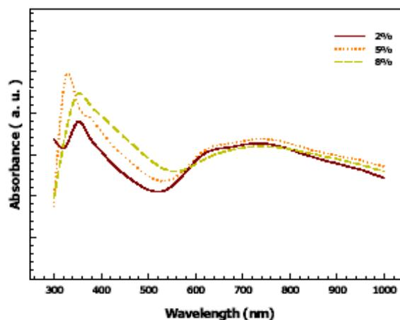
Figure 2. UV-Vis pattern of the various copper loading on the nanosized Cu/ $\gamma$ -Al<sub>2</sub>O<sub>3</sub> catalyst.
