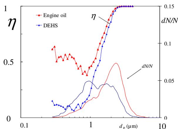
Figure 1. Collection efficiency measurements, for a fixed flow rate of 100 NI/min..
