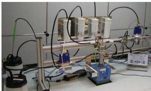
Figure 1. Test-stand for generation of respirable fraction of nano-objects from nanomaterials (vortex shaker method).
