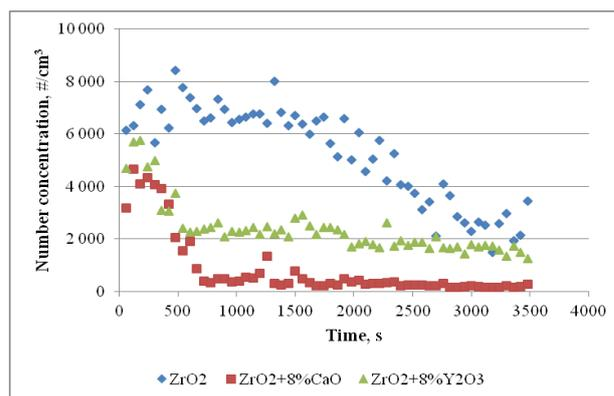
Figure 2. Total number concentration of particles  $0.01-8.14\mu m$  obtained during generation of nanomaterials ( $ZrO_2$ ,  $ZrO_2+8\%CaO$ ,  $ZrO_2+8\%Y_2O_3$ ) with vortex shaker method.
