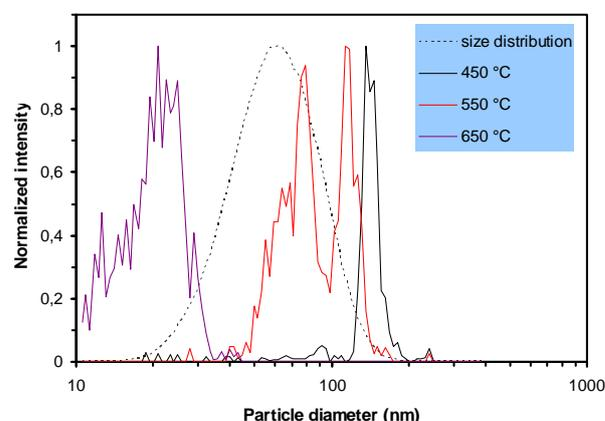
Figure 1. Normalized number size distributions obtained during combustion of wood chips in a 10 MW<sub>th</sub> CFB: total particle size distribution (dotted line), and distributions measured with pre-selected 150 nm particles using the VTDMA setup at three different temperatures (solid lines).
