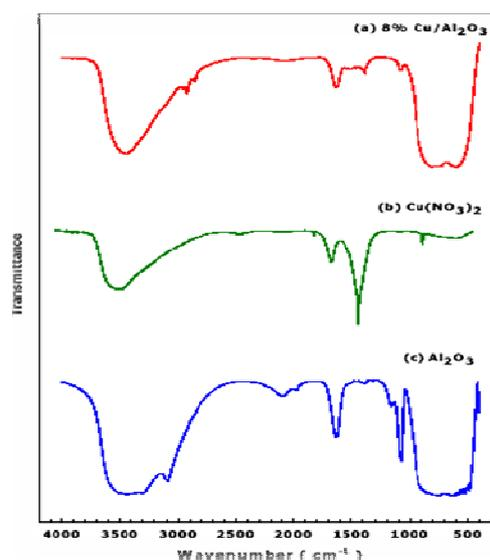
Figure 2. FTIR pattern of fresh nanosized Cu/ $\gamma$ -Al<sub>2</sub>O<sub>3</sub> catalyst.
