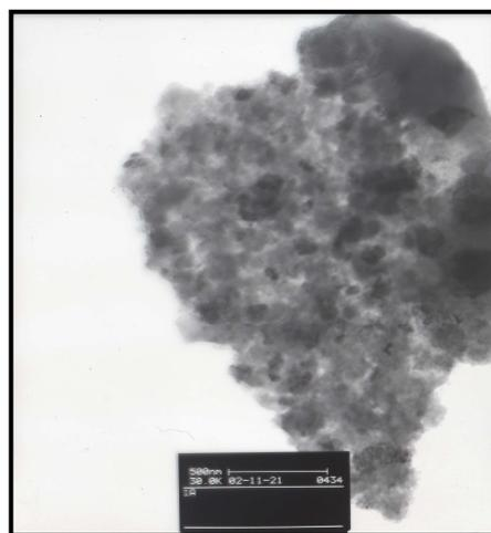
Figure 1. TEM photograph of the fresh nanosized Cu/ $\gamma$ -Al<sub>2</sub>O<sub>3</sub> catalyst.
