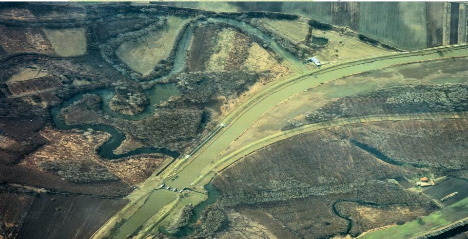
In the 1990s a restoration network was built in all the floodplain forests. It brings water from the rivers back to forests through a system of water channels and sluice gates. The channels are more than 120 km long and the area of new water bodies, periodic and permanent pools covers more than 240 ha.
