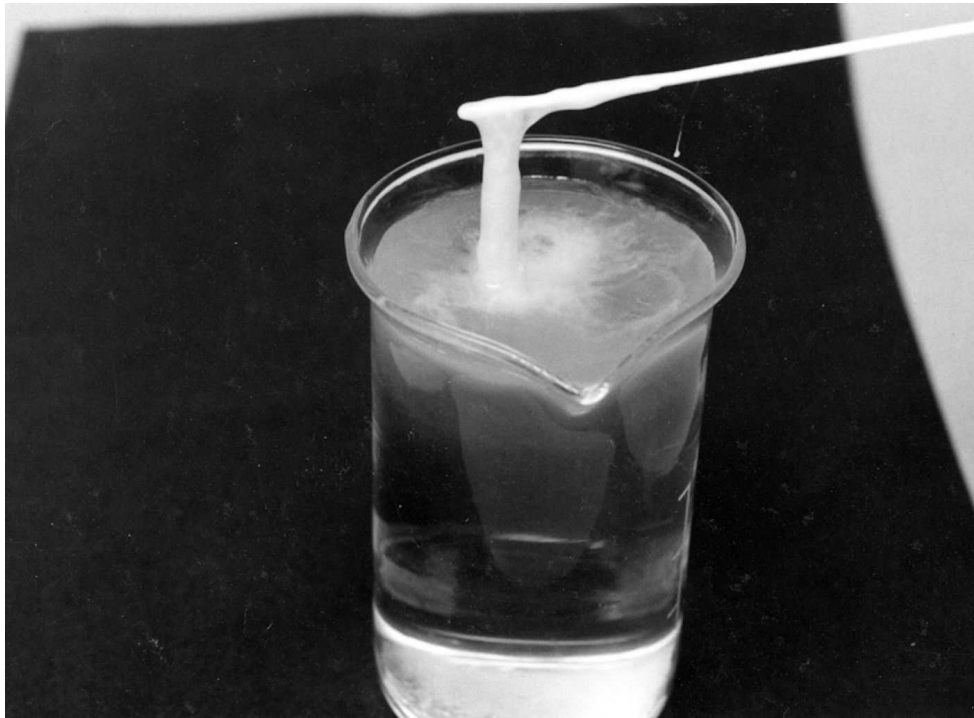
Figure 1: Precipitation of PHEMA injected to water
