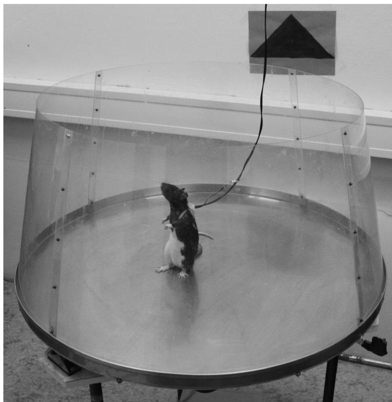
**Figure 1** A photograph of the Carousel apparatus. The apparatus consists of a metallic disk which can be rotated at various speeds and directions. A rat is connected with a wire to the swivel on the ceiling. The wire supplies the LED on the rat and delivers mild footshocks (0.2–0.7 mA).
