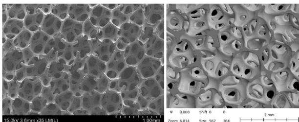
Figure 1. Real structure (left) and generated model (right) of an examined open-pored foam.
