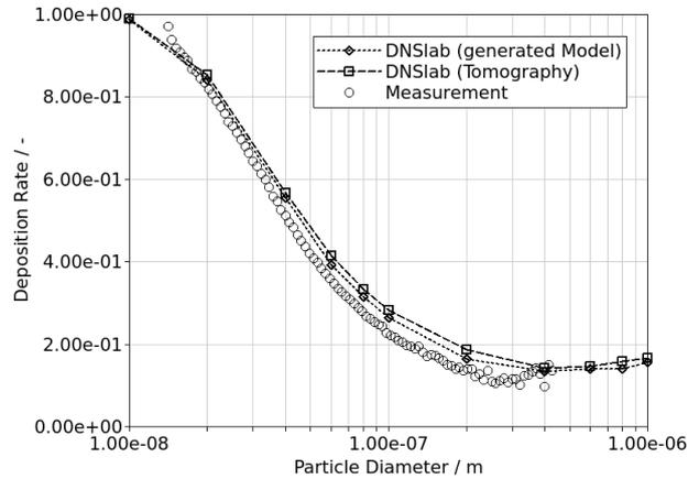
Figure 2. Comparison of NaCl particle fraction deposition rates from experiment and simulation with generated model and tomography for the open-pored foam material shown in Figure 1. The sample thickness is 16 mm, the aerosol flow rate is 0.055 m/s.
