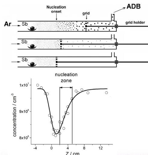
Figure 3. Experimental setup for the "supersaturation cut-off" method and the outlet particle concentration vs. the grid position.
