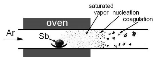
Figure 1. Experimental setup.
