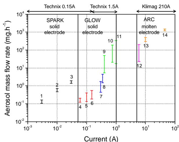
Figure 1. Mass output rate of copper nanoparticles generated by electrical discharges.
