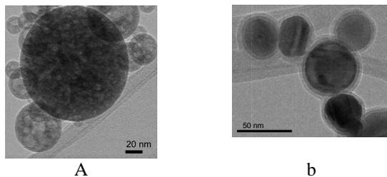
Figure 1: TEM image of (a) iron oxide particles from Fe(NO<sub>3</sub>)<sub>3</sub> precursor (b) iron particles from industrial by-product derived precursor.
