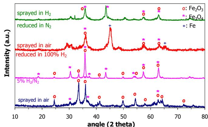
Figure 2. XRD patterns of ASP particles under different spraying and post treatment gas environments.
