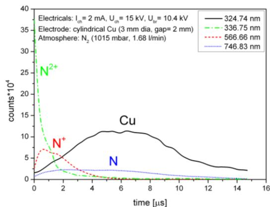
Figure 1. Temporal evolution of the emission of the species detected in the spark discharge.
