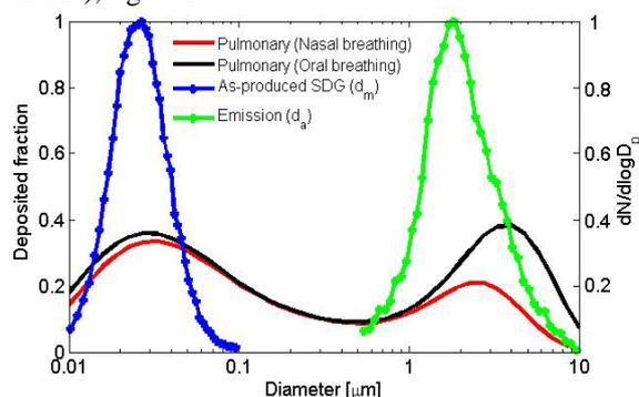
Figure 2. Two pulmonary deposition curves (MPPD) shown together with typical particle number size distributions (normalized) of as-produced particles and emitted particles during maintenance of the generators.
