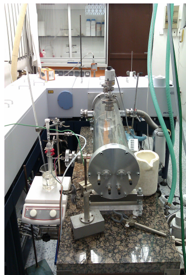
Fig. 1: The multipass cell together with the spectrometer Bruker IFS 125 HR.
