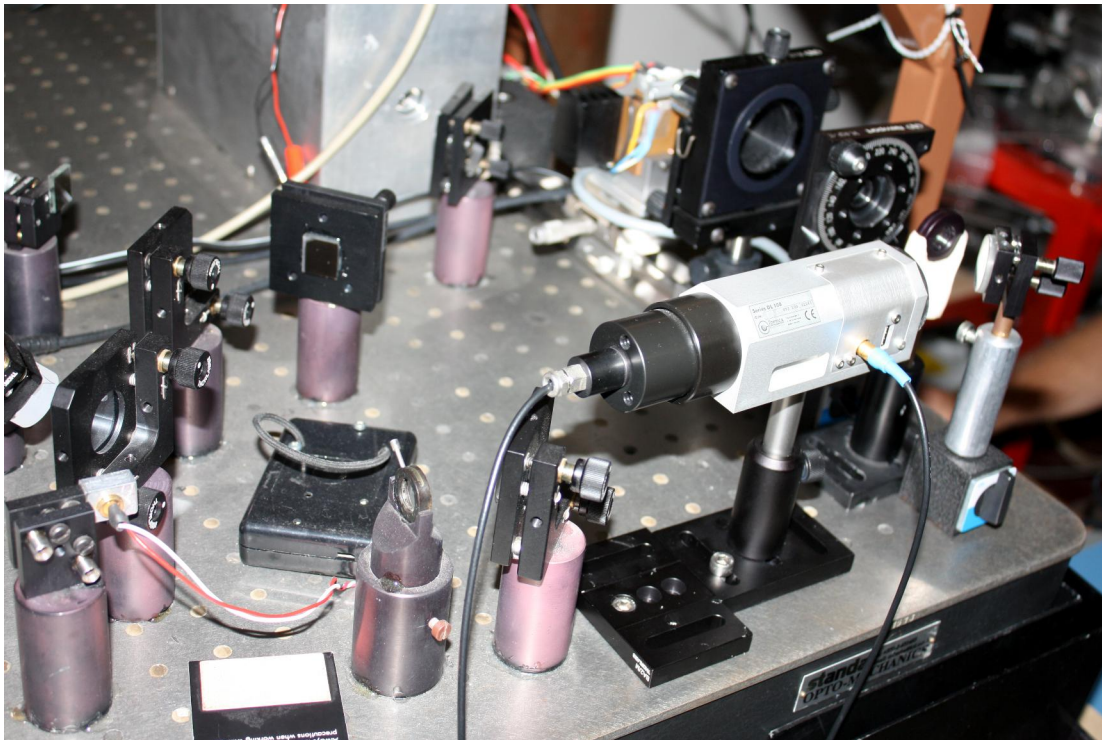
Fig. 10 Measurement setup used for time-resolved high resolution measurements of VCSEL emission spectra
